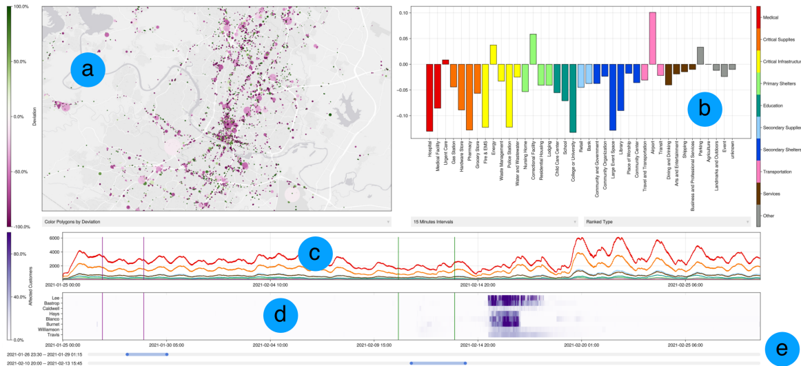
Figure 1: An overview of the MoVis analysis tool (cf. section 4). (a) shows the map with circles that indicate high mobility in specific locations. Users can zoom into the map to see building polygons and display additional information. (b) shows the deviation of movement patterns between two selected time ranges. The colors indicate the category associated with the deviation of a specific type. (c) shows the number of travels over time for each category (d) displays the temporal outage severity for previously selected counties relevant to the study. (e) shows sliders that allow the user to select time ranges for comparison. The selected ranges are shown in (c) and (d) as purple and green vertical line pairs.
