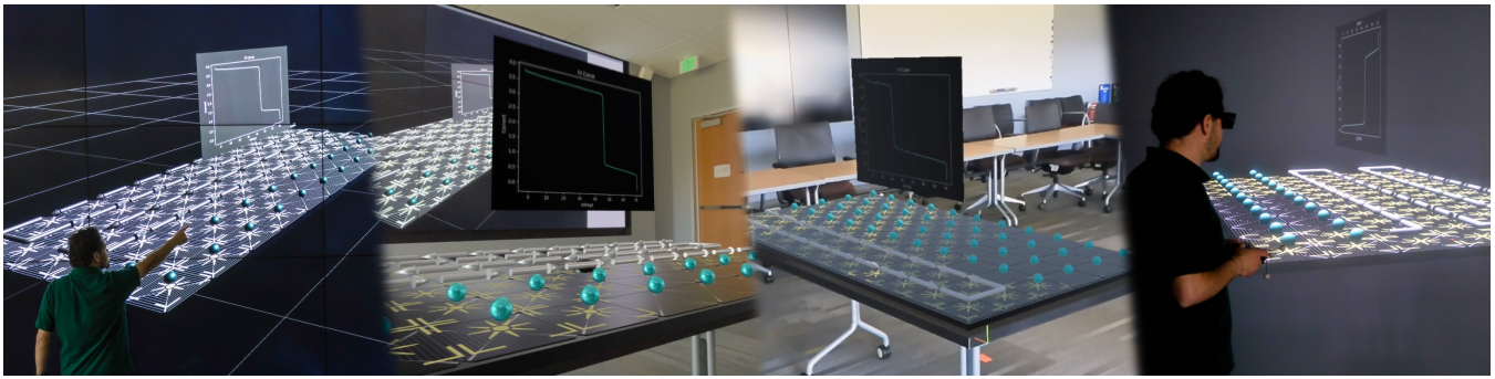
Figure 4: Captures of the system in action on a variety of participant platforms. From left to right; web interface for projection of scene on large-scale displays, Apple Vision Pro with situated visualization, Magic Leap 2 with the same, presentation of scene in an immersive virtual reality environment. Heterogeneity is a key requirement for this system.
