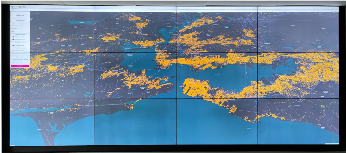
Figure 1: Snapshot of the 100 megapixel high-resolution display with an interactive visualization in the browser. Two synthetic energy model topologies are shown: an electrical transmission system (blue lines) and a corresponding distribution system (orange points) in the San Francisco Bay area. These two models have over 12 million combined features.
