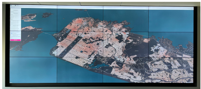
Figure 3: San Francisco SMART-DS model on the Insight Center 100 megapixel display wall. Assets are styled from time-series values with a diverging color-scale based on nominal per-unit voltage (white) and +/-5%, with red as higher and blue as lower voltages.
