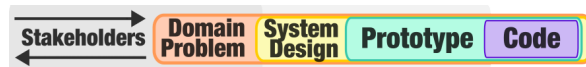
Figure 4: Cartoon of a visualization system broken out into four stages of reflection, following Munzner’s nested model of design and validation [29]. First a decision maker is interviewed by a design practitioner, who solicits a domain problem and identifies a system design which addresses it. Then a visualization developer will create a prototype by writing code to process the dataset. To evaluate the results, a domain expert will use the prototype to explain how the dataset addresses the problem, while in conversation with a design practitioner. This typically reveals both technical issues requiring the visualization developer to update the code, and conceptual issues requiring the design practitioner to update the prototype description. Ideally this process will repeat until the stakeholders are both satisfied with the system, and it addresses their actual problem.
