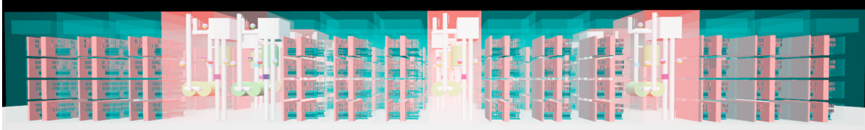
Figure 1: Prototype of the Frontier digital twin using Unreal Engine 5. All child components are visible: The first row, shows 12 compute racks and four cooling distribution units 1 . The racks show, among others: cable trays, rectifiers 1 , and compute nodes, with all CPUs, GPUs 1 and DIMMs visible. ( 1 : Colored according to power consumption.) Total actors: 152,906.
