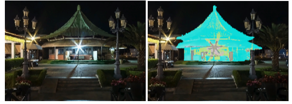
Figure 3: As different environment pixels can have the same most perceptually distant color, computing a per-pixel most distant color results in “clumping”, the loss of the background details as in the image on the right.
