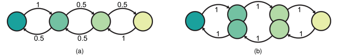
Fig. 3: (a) Example of a plain Markov chain strategy. The probability of going from left to right without returning is 25 %. (b) In the expanded version, where the patrol retains memory, the probability is 100 %.
