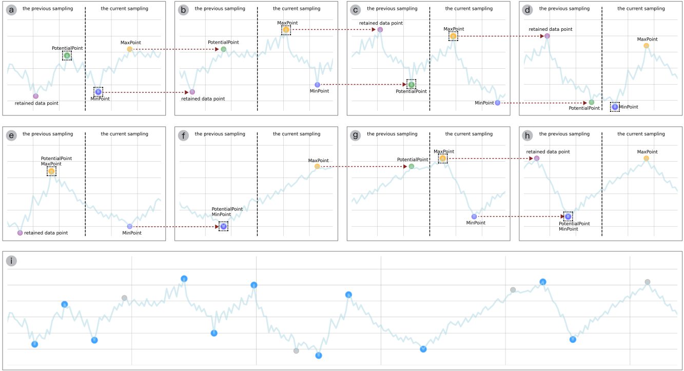
Fig. 2: Figures a through h illustrate the sampling process of 270 data points at a sampling ratio of 30 : 1. In each image, the data points to be retained in the current sampling are framed with a black dashed rectangle. Between adjacent images, "the current sampling" of the preceding image is "the previous sampling" of the following image. Dashed arrows show the updating process of variables. Figure i is the image formed by connecting Figures a through h , showing the final sampling effect of 270 data points, with a total of 11 data points highlighted in blue that were retained.
