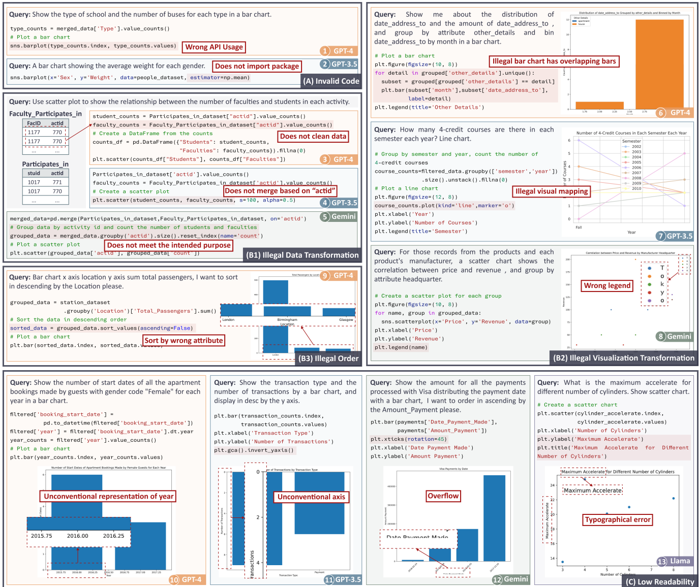
Fig. 11: Typical errors: (A) pertains to invalid code error. (B1-3) denote illegal errors occurring during data transformation, visualization transformation, and sorting processes. (C) relates to issues of low readability.
