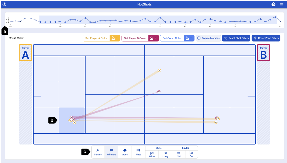
Figure 1: The HOTSHOTS Tennis Visualization System. We visualize stroke-by-stroke tennis data on a visual representation of the court. Filter allows for limiting the strokes to be shown: (a) in time, (b) in space, and (c) by stroke type (net, out, win, serve, etc).
