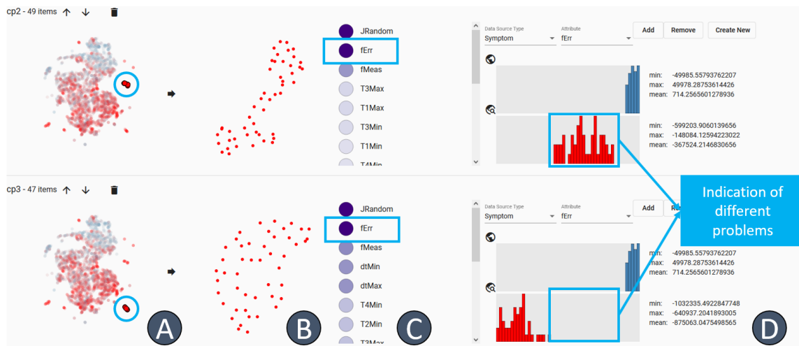
Figure 6: The Refine view allows investigating and modifying clusters of interest that are visualized in a row-based layout for easier comparison. This example shows two clusters mainly comprising failed test cases (in red). For each row, The scatter plot (A) highlights the respective cluster on the initial global projection based on symptoms (first phase). The second scatter plot (B) visualizes the reprojection of the respective data selection to help understand potential intra-cluster patterns. Column (C) shows a ranking of interesting attributes based on the Kolmogorov–Smirnov test. The histogram views (D) show how the distribution of values of a specified attribute differs between a reference cluster (top histogram in each row) and the respective clusters (bottom histogram), which helps delineate different subproblems.
