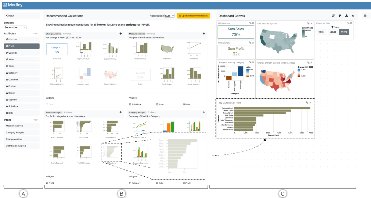
Fig. 1. MEDLEY’s user interface. (A) Data attribute and intent input panel, (B) collection recommendation zone, and (C) dashboard canvas. Views and widgets added to the canvas are faded out in the recommendation zone.
