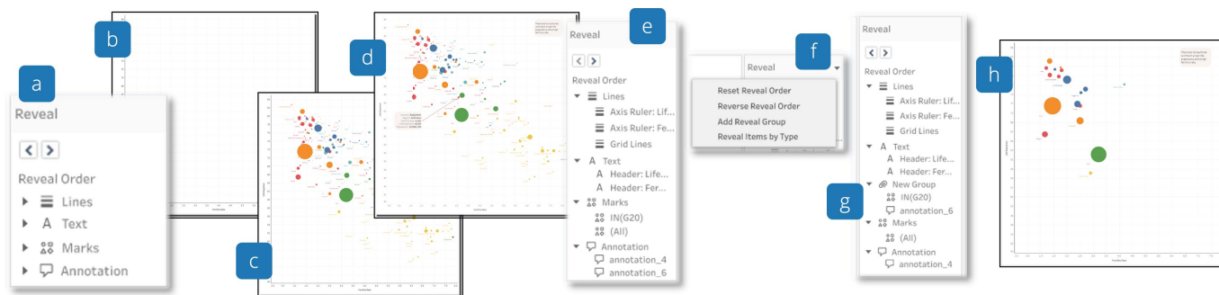
Fig. 1. This example from the progressive reveal design probe demonstrates the reveal of a scatterplot. A reveal control interface (a) indicates an initial ordering of lines & axes (b), marks (c), and annotations (d). This ordering can be expanded (e), appended to with a new reveal group (f), and reordered (g), resulting in a new sequence that interleaves marks and annotation (h) before arriving at the final reveal state (d).
